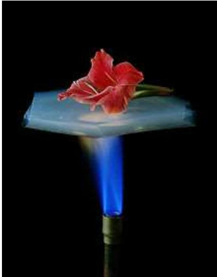
A flower is on a piece of aerogel which is suspended over a flame from a [Bunsen burner](#). Aerogel has excellent insulating properties, and the flower is protected from the flame.
