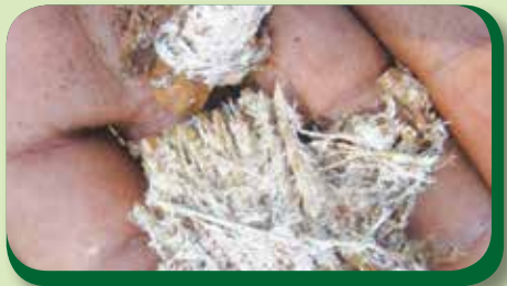
Fibers of asbestos found on the soil
